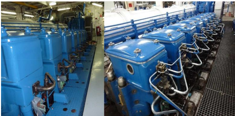
Figure 2.14: Methanol engine before and after conversion (Source: Wartsila)
