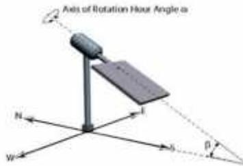
**Gambar 2.1** *One Axis Tracking*
