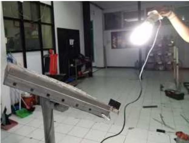
**Gambar 4.3** Rangkaian peralatan validasi sensor
