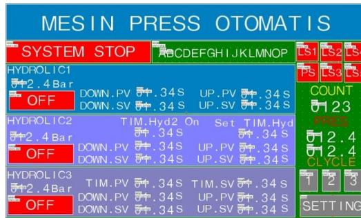
**Gambar 3.8.** Tampilan control *press machine*.
