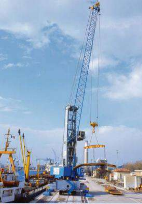
Gambar 19 Harbour Mobile Crane HMK 260
