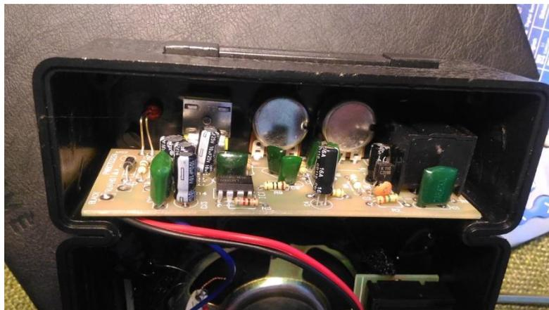
Gambar 2. 16 Komponen Mini amplifier Marshall MS-2
