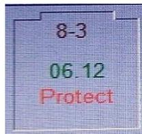
Gambar 4.16 Kondisi *Protect* Di Pengujian *8-Channel Battery Analyzer*
