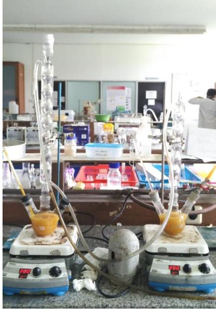
Gambar 4.5 Rangkaian refluks sintesis biodiesel
