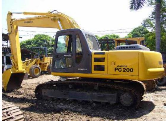
Gambar 3.2. Excavator Backhoe merk KOMATSU
