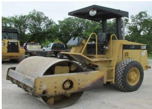
Gambar 3.4. *Vibration Roller* Caterpillar
