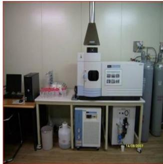
**Gambar 3.4** Mesin OES (*Optical Emission Spectroscopy*)
