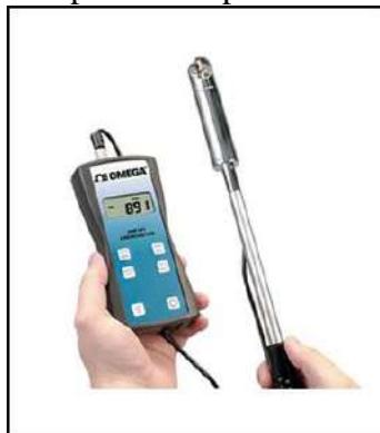
*Gambar 3.9 Anemometer Omega HHF141*
