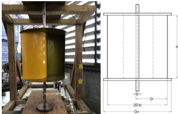
**Gambar 3.5 Turbin Angin Savonius**
