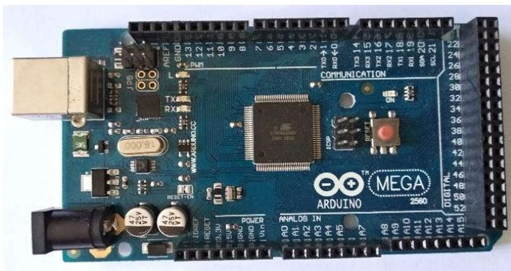
**Gambar 2.3 Arduino Mega 2560**
