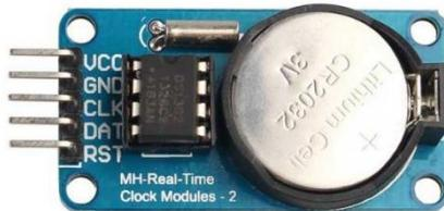
**Gambar 2.10 RTC (Real Time Clock)**
