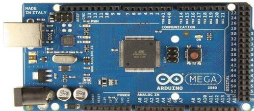
**Gambar 2.8.** Board *Arduino Mega 2560*
