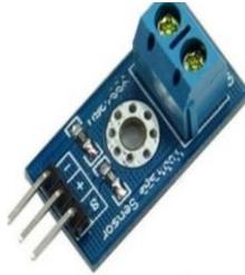
Gambar 3.12 Modul sensor tegangan *voltage divider*
