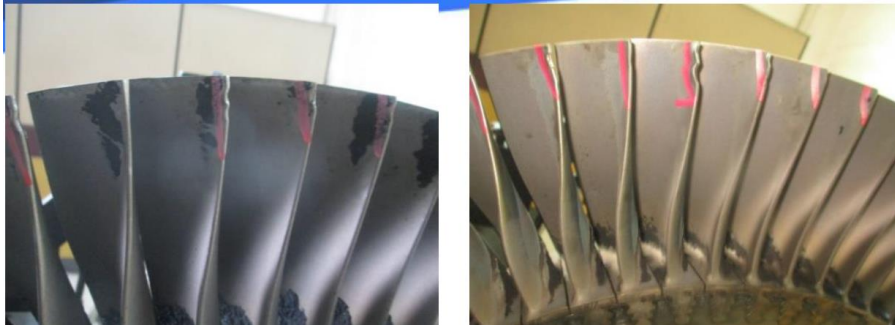
Figure 1. 2 Damaged turbine side of turbocharger (Source: Samudera Indonesia Ship Management)
