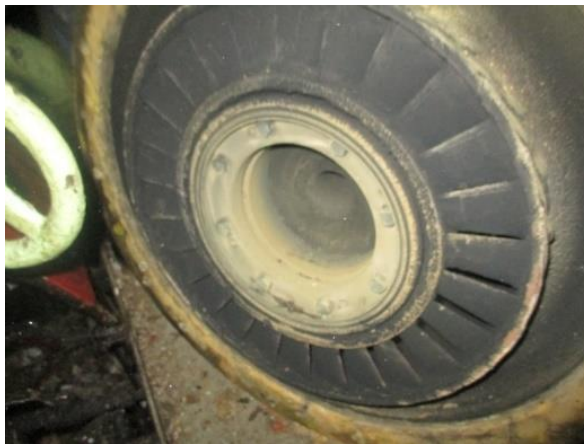
Figure 2. 7 Carbon Deposits on Nozzle Ring (Source: Samudera Indonesia Ship Management)
