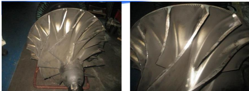
Figure 1. 1 Damaged compressor side of turbocharger (Source: Samudera Indonesia Ship Management)
