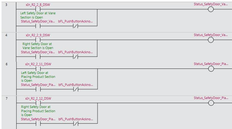
**Gambar 4. 12** Program *Error vane dan placing section safety door contact*
