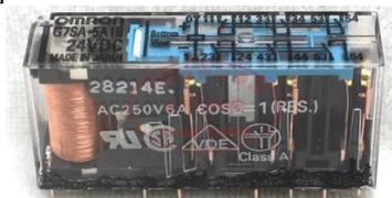
**Gambar 2.9** Tampilan fisik *safety relay* G7SA-5A1B [13]
