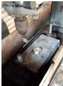
Gambar 3.28 Proses Machining Fix plate
