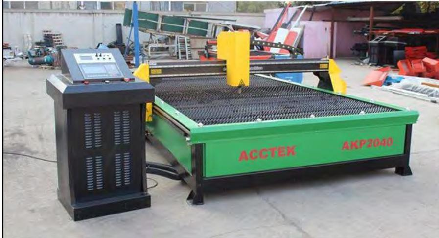
Gambar 5.7 Mesin CNC Cutting
