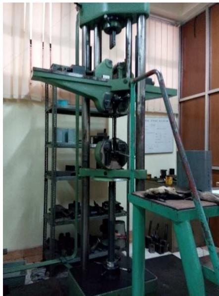
Gambar 3.9 *Universal Testing Machine* (UTM) berkapasitas 200 kN
