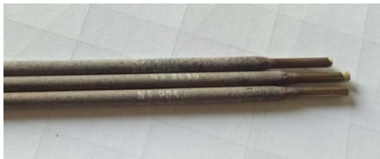
Gambar 3.7 Filler NS 9050 diameter 3,2 mm
