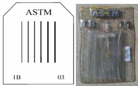
Gambar 2.26 Wire image quality indicator
