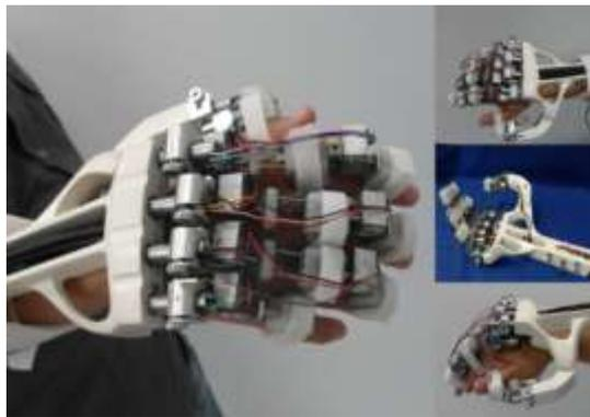
Gambar 1.5 Precision Grip Eksoskeleton
