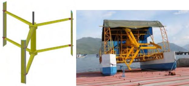
Gambar 4.20 Prototype turbin arus laut type darrieus
