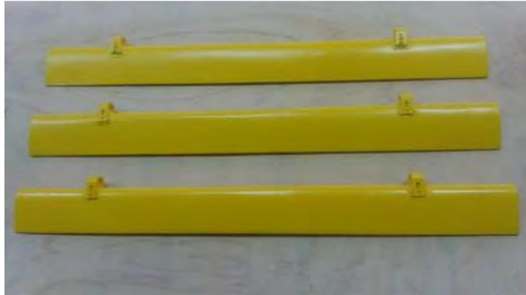
Gambar 3.4 *Darrieus turbine blade type aerofoil naca 0021*
