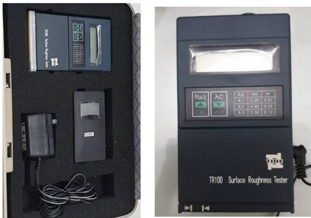
Gambar 3.12 Alat TR100/TR101 *Surface Roughness Tester*
