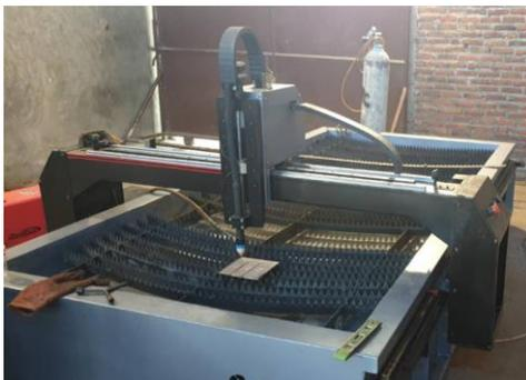
Gambar 3.4 Mesin CNC *Plasma Cutting* Hyspeed HT2000
