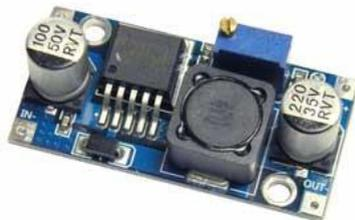
**Gambar 2.5** DC-DC Converter
