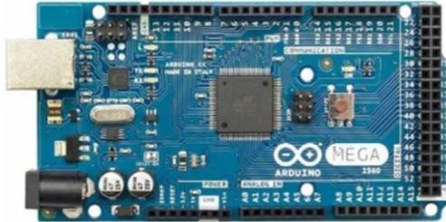
**Gambar 2.7** Arduino Mega
