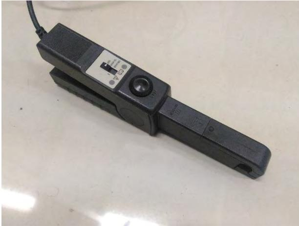
**Gambar 3.16** Current Probe Tektronix A622
