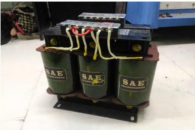
**Gambar 3.3** Transformator 3 kVA 3 fasa
