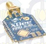
**Gambar 3.4** Modul Xbee Pro S3B
