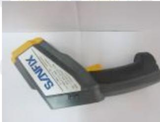
**Gambar 3.5 Termometer Infrared**
