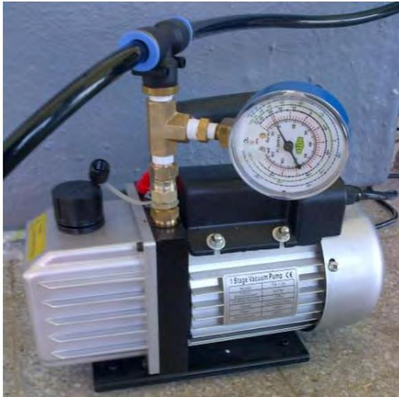
Gambar 4.3. Pompa Vakum
