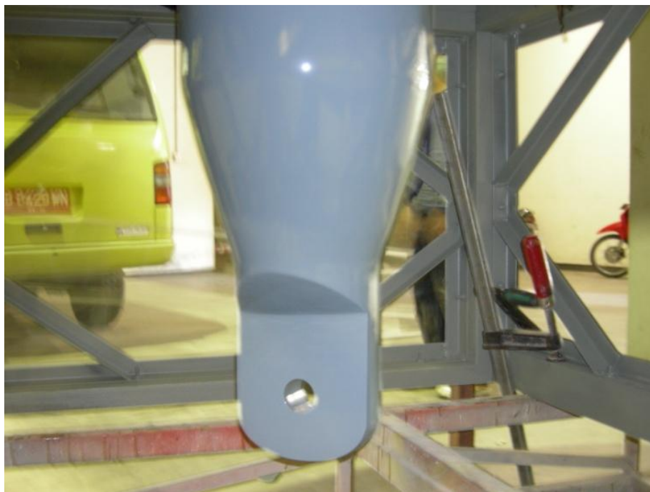
Figure 3: Keel structure of the tsunami buoy [2].
