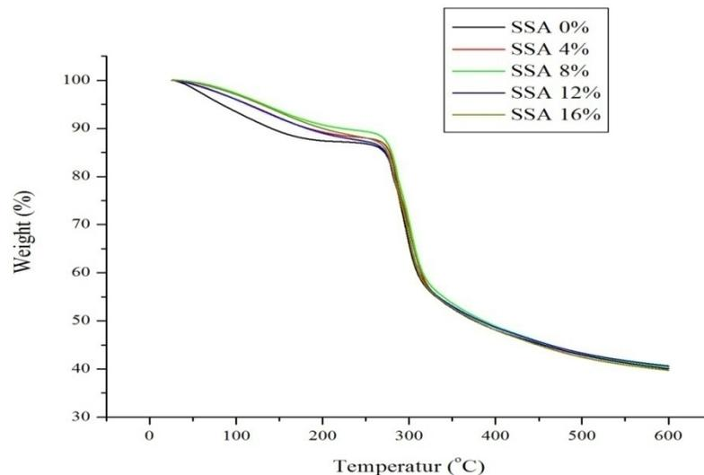
Figure 1. Thermograms of CS/MMT-Sil 10% and CS/MMT-Sil 10%/SSA membranes
