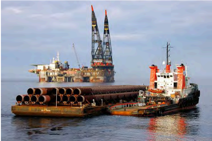
Gambar 8.3 Transport Tiang Pancang
