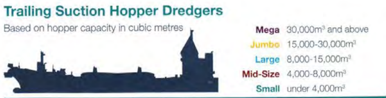
Gambar 2.14 Ukuran TSHD Berdasarkan Kapasitas Hopper ( sumber: International Association of Dredging Companies )
