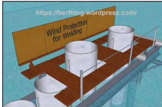
Gambar 8.5 Pemotongan Steel Pipe Sheet Pile (sumber: berthing.wordpress.com )
