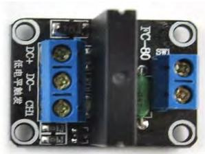
**Gambar 4.6** Modul SSR 1 *channel*
