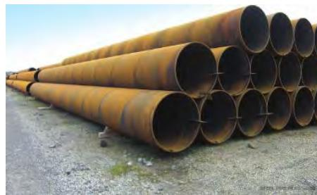
Gambar 2.2 *Steel Pipe Pile*
