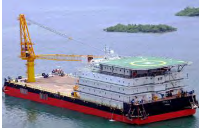
Gambar 2.10 Accommodation Work Barge (Sumber: https://ottomarine.com )
