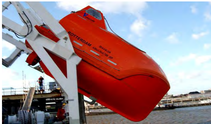
Gambar 2.26 Freefall lifeboat (Sumber: https://vanguardlifeboats.com )
