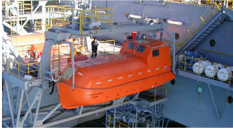
Gambar 2.25 Davit-operated lifeboats (Sumber: https://nauticexpo.com )
