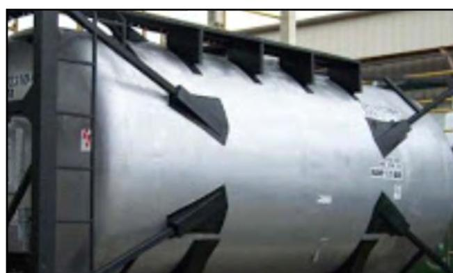
Gambar 5. ISO-Tank Container IMO-2
