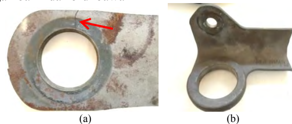
Gambar.4.(a) Kerusakan outer link chain ; (b) Kerusakan mounting angle
