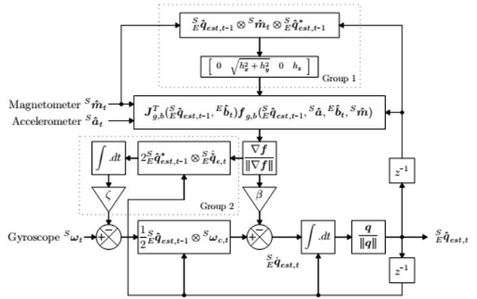
Gambar II Diagram Blok Algoritma AHRS Madgwick
