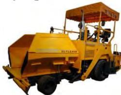
Gambar 2.23 Asphalt finisher
