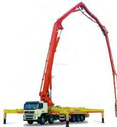
Gambar 2.20 Concrete Pump
