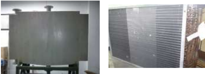
Gambar 2.3 hasil rancangan kondensor shell and tube dan evaporator tipe compact
