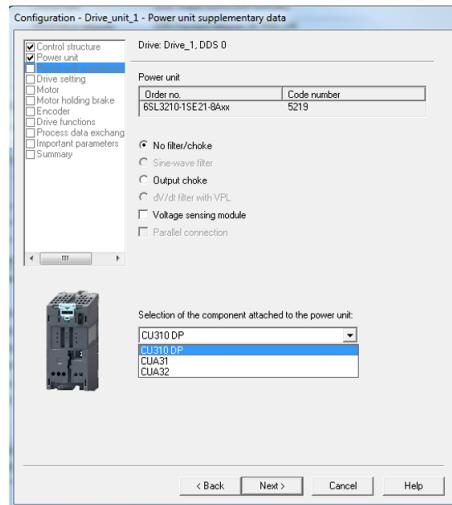
Gambar 3. 29 Pilih *Power Unit Supplement*
