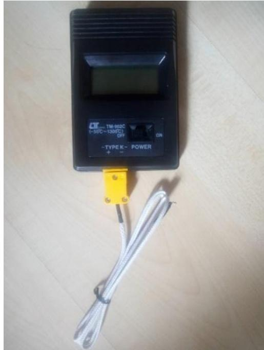
**Gambar 4. 6.** Instrumen Termometer Digital
