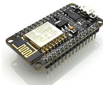
**Gambar 3. 6 NodeMCU ESP8266**
