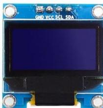
**Gambar 3. 8** OLED Display SSD1306 0.96” inch White
