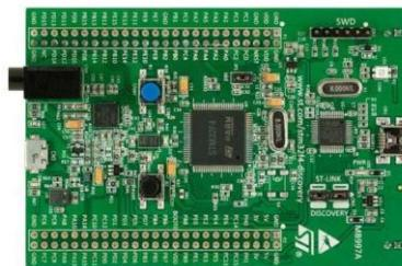
**Gambar 2.13** Mikrokontroler STM32F4 *Discovery*
