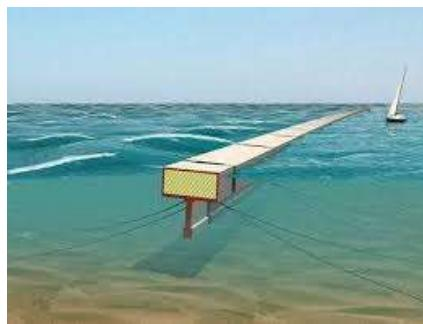
**Gambar 2.1. Floating Breakwater**
