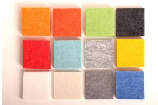
Gambar 4.23 *Polyethylene Terephthalate*
