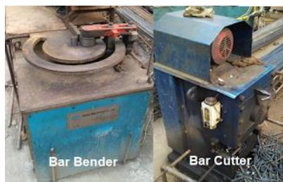
**Gambar 4.50.** Bar Bender dan Bar Cutter
