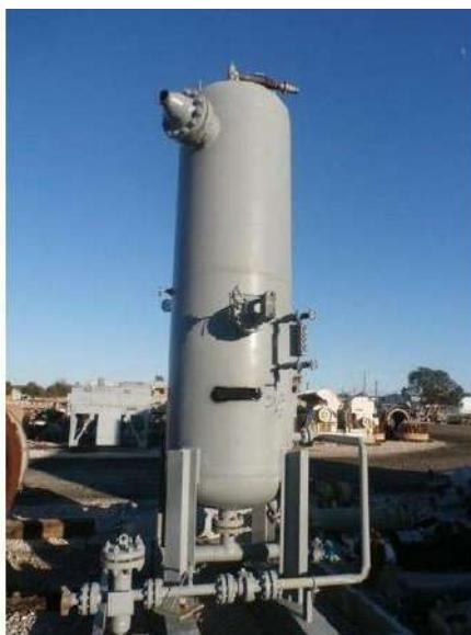
**Gambar 2.3 Pressure Vessel Vertikal**
