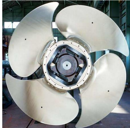
Gambar 2. 4 *Controllable pitch propeller*
