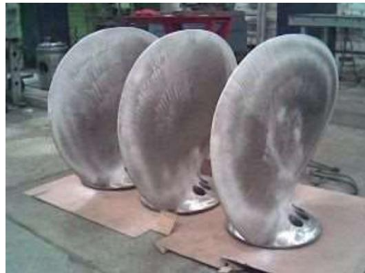
Gambar 2. 3 *Blade Controllable pitch propeller*
