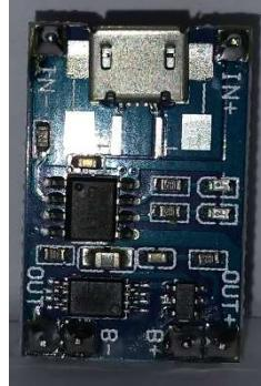
Gambar 2.20 *Charge Controller TP4056*
