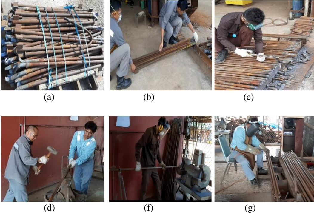
**Gambar 1.3 Proses *repair puncher bar***
